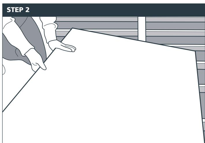
Install the first panel following guidelines and best practices, including fixings centres and types. The fixings heads should be flush or just below the panel surface.
