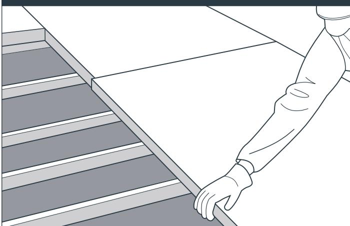
Continue installing the panels as required in a staggered pattern by repeating the fixing, gluing and taping steps for each panel.
