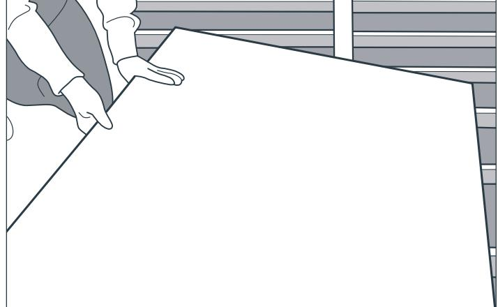
Install the first panel following guidelines and best practices, including fixings centres and types. The fixings heads should be flush or just below the panel surface.
