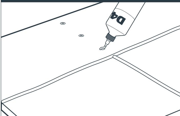
Fixing heads should be sealed by applying a bead/drop of D4 rated (EN 204) foaming adhesive.
