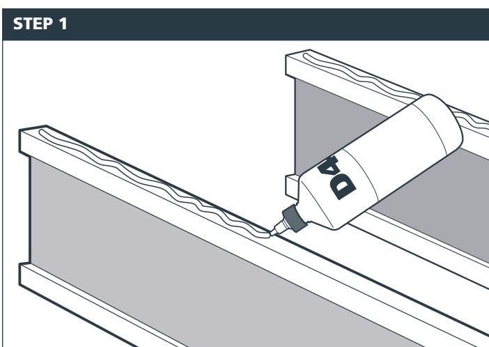
Apply one continuous bead of D4 rated (EN 204) adhesive to the top of the joists and noggins corresponding to the area of the 1st panel to be installed.
