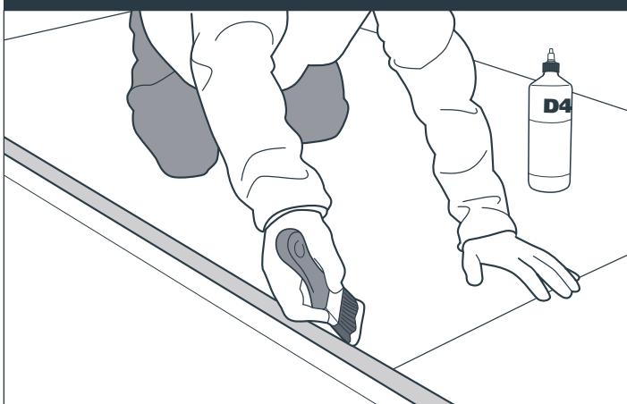
All exposed edges should be sealed by applying a continuous layer of D4 rated (EN 204) adhesive by using a brush or by wrapping a specialist waterproof high-performance polyethylene-coated cloth tape around the edges.
