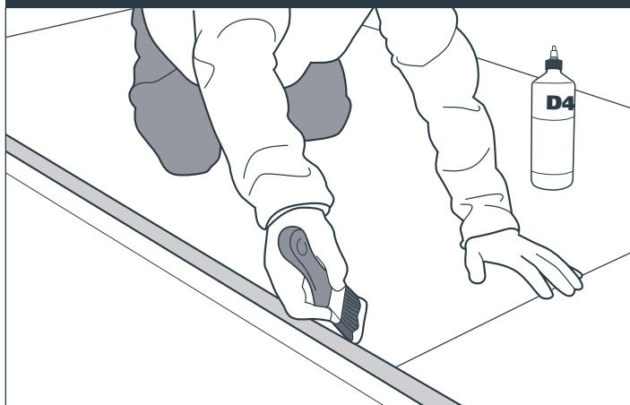
All exposed edges should be sealed by applying a continuous layer of D4 rated (EN 204) foaming adhesive by using a brush.
