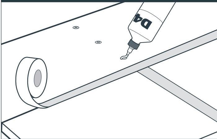
Fixing heads should be sealed by applying a bead/drop of D4 rated (EN 204) adhesive or by tape.
