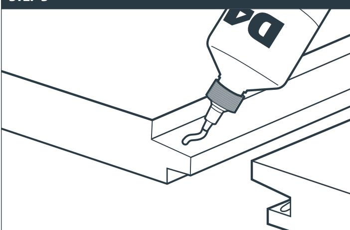
Apply one bead of D4 rated (EN 204) foaming adhesive on both the tongue and groove of the joints about to be installed making sure that the entire joint is bonded. The adhesive should foam out of the joints on the panel surface once installed to help seal the joint and prevent water ingress and edge swelling.
