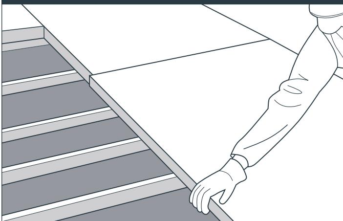
Continue installing the panels as required in a staggered pattern by repeating the gluing and fixing steps for each panel.
