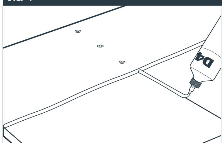
Apply one bead of D4 rated (EN 204) foaming adhesive on the cut edges on top of the joists allowing the adhesive to foam out on the panel surface to help seal the joint and prevent water ingress and edge swelling.
