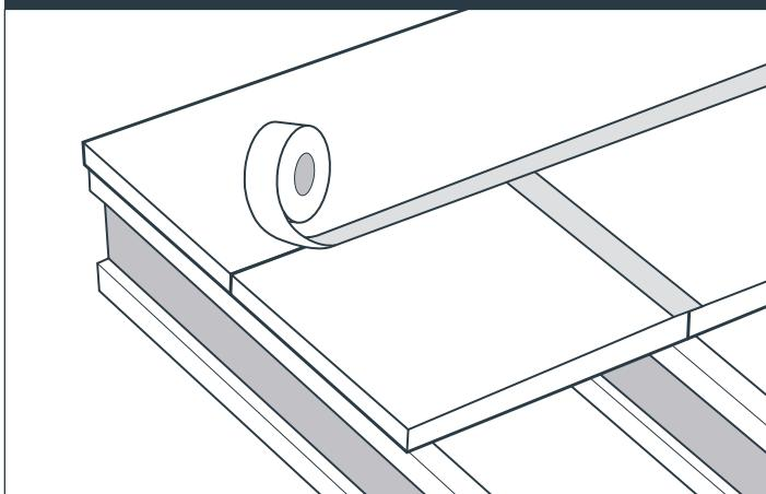
All floor joints should be sealed and protected with a specialist waterproof high-performance polyethylene-coated cloth tape. This will prevent moisture ingress in the panel edge and edge swelling.
